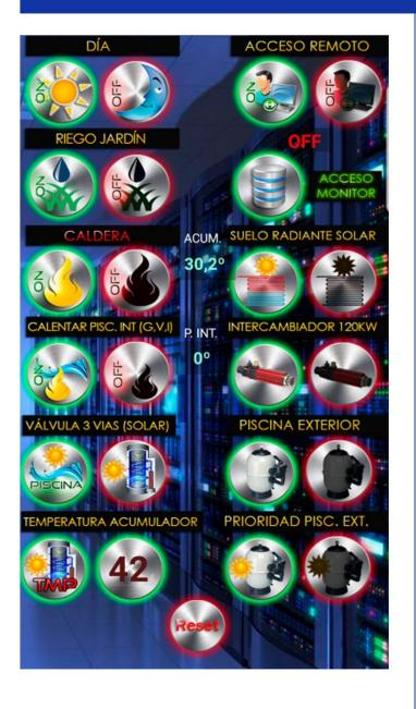
From this screen you can control the irrigation although it does it automatically according to the weather forecast. The boiler temperature and the possibility of heating indoor pool with gas.
