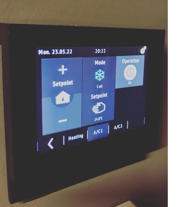
Using the adequate KNX gateway the user can control the VRV system via KNX touch panels on the wall or even via the KNX server application.
